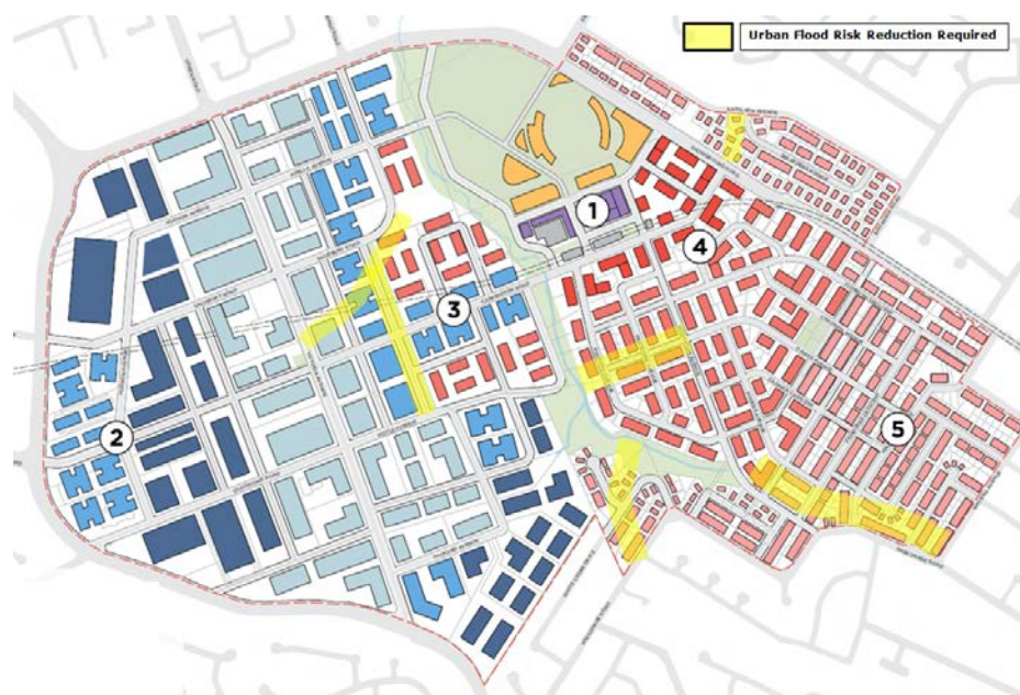
Figure 16 Showground Station Precinct Proposed built form diagram highlighted to show priority overland flowpaths
